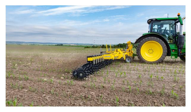
Whether you are cultivate the land in conventional or organic farming, this machine is perfect for you. Its agronomic use offers, for example, crushing of soil crust, soil aeration, mechanical disposal of shallow-growing weeds, stubble cultivation, incorporation of mineral fertilisers, plant growth promotion and interruption of capillarity.
